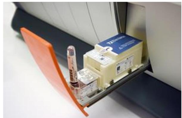
The T2Bacteria Panel is placed into the T2Dx Instrument to identify sepsis-causing bacteria
